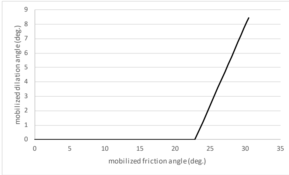
Figure 27. Mobilized dilation angle \psi_m versus mobilized friction angle \phi'_m for peak friction and dilation angles of 30^\circ and 8^\circ , respectively, and cohesion of 8 kPa.
