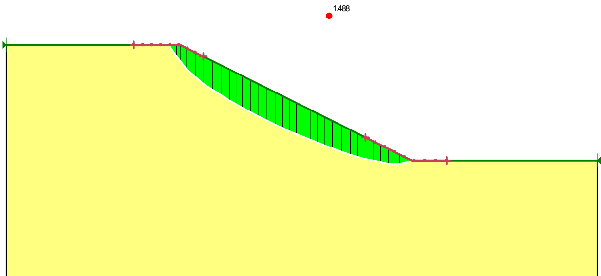
Figure 6. Factor of safety based on Limit Equilibrium stability Analysis.
