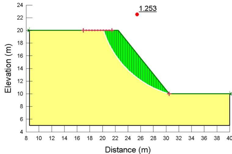
Figure 5. Critical slip surface and factor of safety with no tension crack (Analysis 1).
