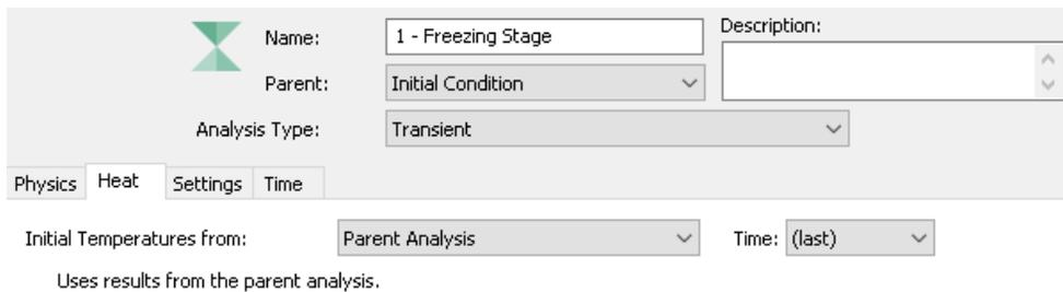
Figure 3. Initial temperatures used from the Parent analysis in the Heat tab.
