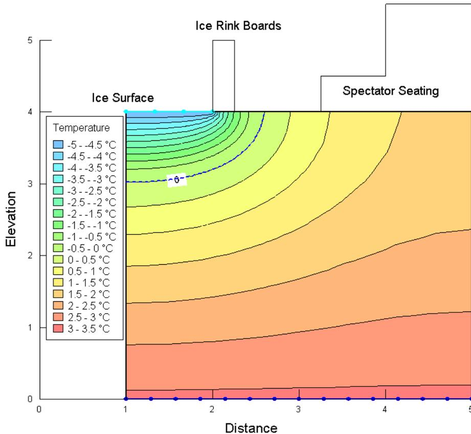
Figure 8. Freezing front location after 100 days.
