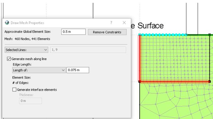
Figure 6. Mesh refinement of the soil region directly below the ice.
