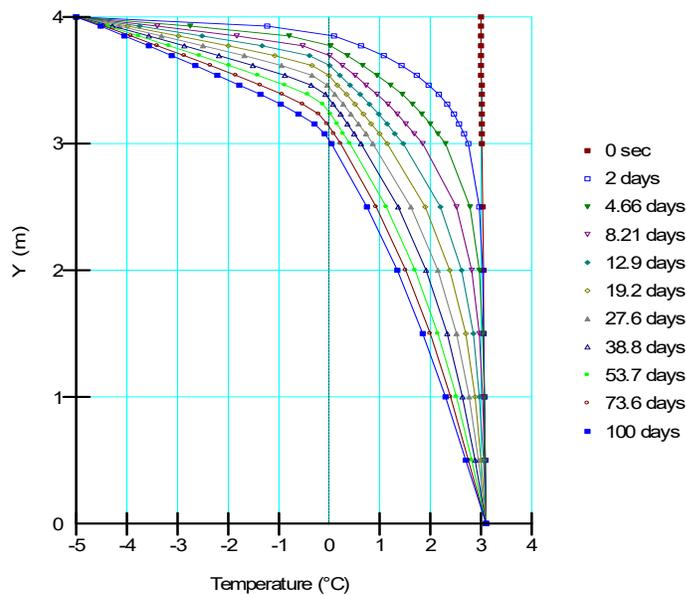
Figure 10. Ground temperature profiles at the left edge of the domain.
