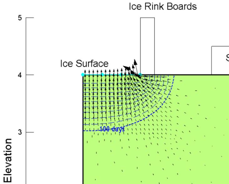
Figure 9. Freezing front location with each time step.
