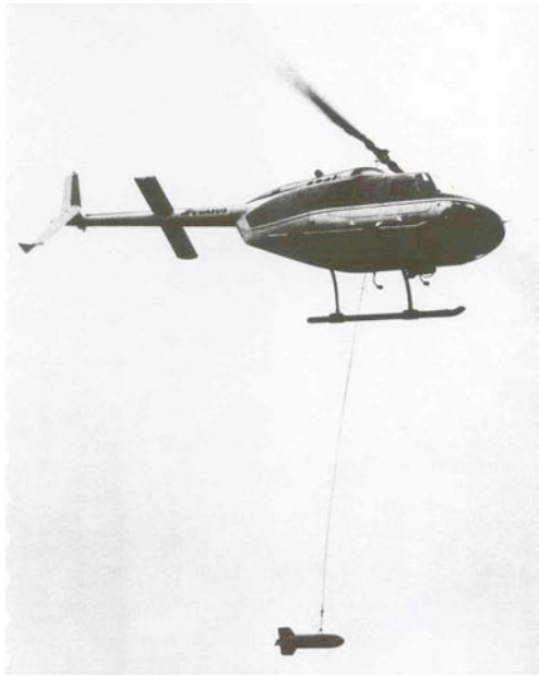
Figure 3.3 Left, a magnetometer slung below a helicopter as a 'bird' installation and, right, a magnetometer in a 'stinger' behind a fixed-wing aircraft.
