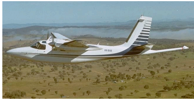
Figure 3.3 Left, a magnetometer slung below a helicopter as a 'bird' installation and, right, a magnetometer in a 'stinger' behind a fixed-wing aircraft.
