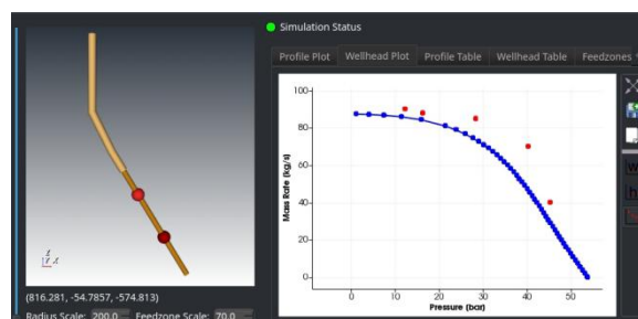
Figure 5: The Gudrun standalone GUI for the Volsung wellbore simulator. The screenshot depicts a deliverability curve on the right and a deviated well with its casing configuration and feedzone locations displayed in 3D on the left.
