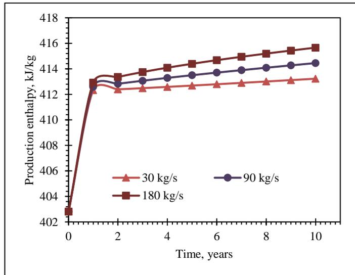
**Figure 6. Simulated average enthalpy change over the production time of 10 years for the field showing three different total production rates.**
