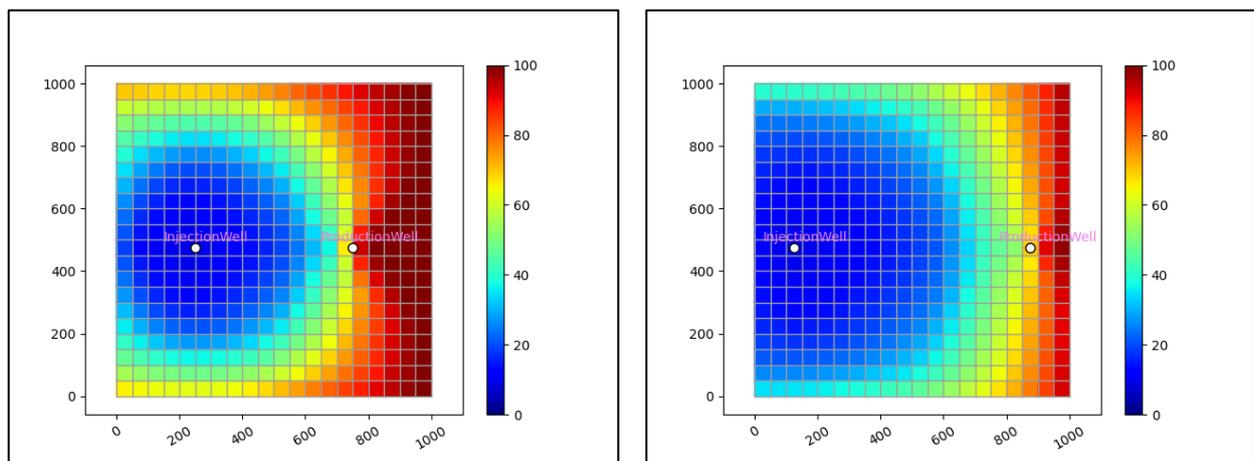
**(a) Horizontal slice of the reservoir temperature distribution at a depth of 130 m after 10 years for 220 kg/s production rate for a 500 m separation between the wells.**
