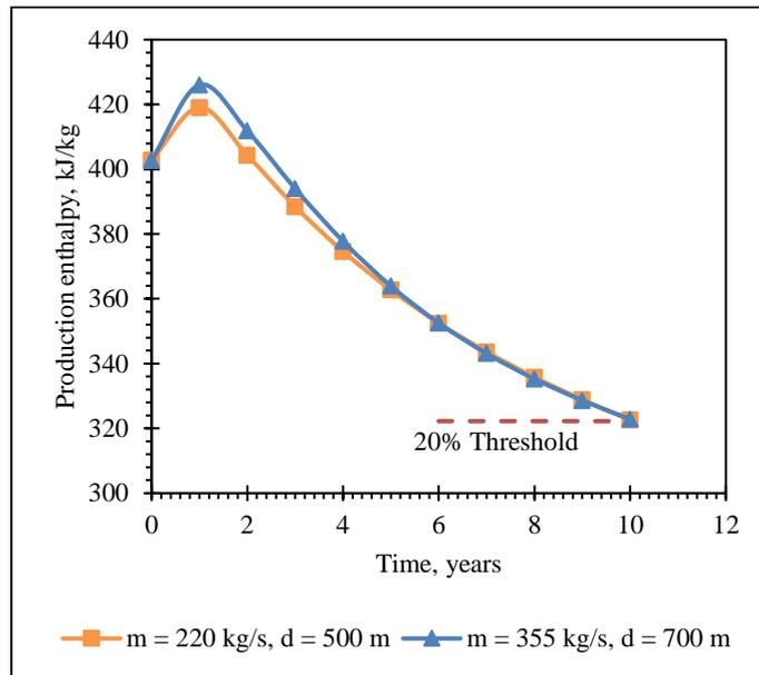
Figure 4. Decline in production enthalpy with respect to time for 220 kg/s and 355 kg/s production rate after 10 years for 500 m and 700 m apart wells, respectively.
