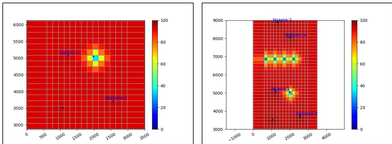
**(a) Horizontal slice of the reservoir temperature distribution at a depth of 180 m after 10 years for 30 kg/s total production rate in the field.**
