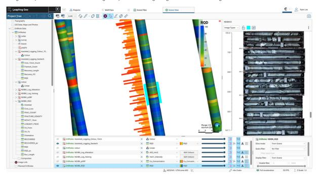
The integrated Imago panel streams images from the cloud directly within Leapfrog without needing to open any external links. Multiple imagery types can be visualised and compared at the same time, including wet and dry core photos or hyperspectral images and mineral maps from core scanning. The in-scene highlight provides spatial context to the imagery as it is being viewed. The highlight visibility can be customised in several ways including scale, opacity, colour, and visibility.
