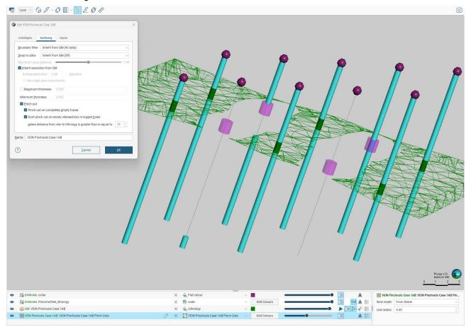
A small yet important update to the vein modelling tool allows pinch-outs on empty intersections that occur in otherwise logged holes. An additional option has been added to the surfacing tab of the editing dialog so that you can control if/when you invoke a change to your modelling strategy. No changes will be enforced to existing vein models.
