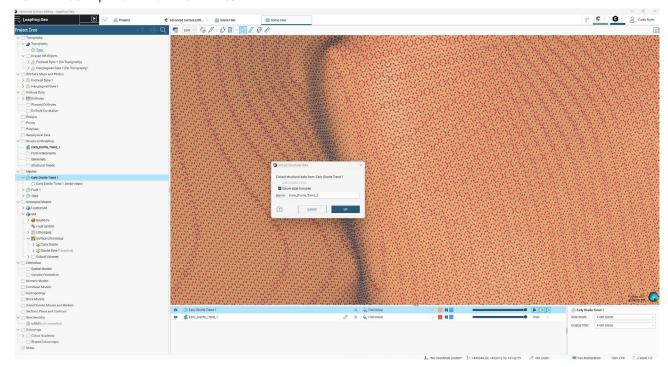
A new "Extract Structural Data" workflow generates a structural measurement (dip and azimuth) for every triangle in a mesh, directly. This omits the need to first extract vertices and subsequently "Estimate Structural Data" (note that the existing "Estimate Structural Data" functionality has been retained).
