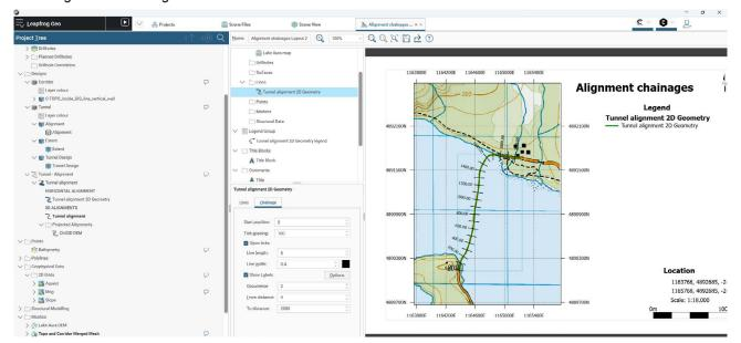
Alignment chainage can now be displayed on Plan Views and/or Cross Sections. This will improve understanding and communication about relative positions along alignments on the plan, cross section, and in the 3D scene.
