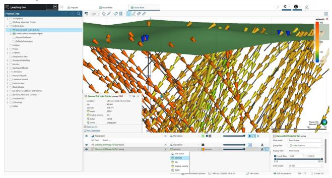
Hole orientation information from downhole surveys is critical to determining the path of a drillhole. Survey data locations can now be visualised in the 3D scene as orientated cones, providing rapid visualisation and validation. Cones can be coloured by azimuth, dip and dogleg severity using the same colourmap and labels display options available as for any other type of data. Scene filtering on the display or selected column allows for optimal flexibility when viewing the data in 3D.
