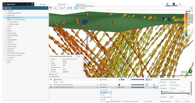
Hole orientation information from downhole surveys is critical to determining the path of a drillhole. Survey data locations can now be visualised in the 3D scene as orientated cones, providing rapid visualisation and validation. Cones can be coloured by azimuth, dip and dogleg severity using the same colourmap and labels display options available as for any other type of data. Scene filtering on the display or selected column allows for optimal flexibility when viewing the data in 3D.
