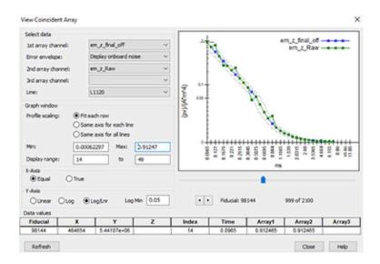
The EM Utilities extension for Oasis montaj provides essential tools for inspecting TDEM arrays, performing Tau calculations, filtering and removing noise.
