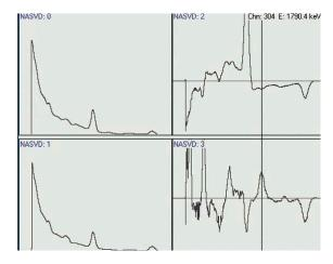
Higher order components can be explained as mixed nuclide responses collected at average survey altitude. They are followed by components that account for the altitude changes. The remaining components contain statistical and instrumental noise.
