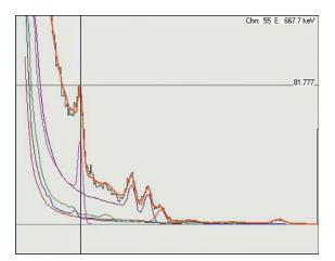
New model responses allow for the contribution of the secondary radiation and for the peak resolution to fit characteristics of the real spectrometer system. Using these detector responses, Praga3 is able to process spectrum information from 0.2 to 3.0 MeV. Background removal for aircraft, cosmic and radon background components can be separately adjusted by the user with the control of experimental calibration constants.
