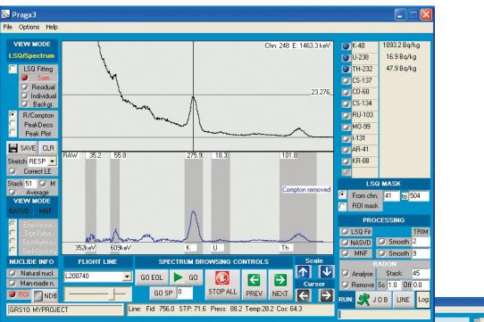
This feature-rich, GUI-oriented software was specifically developed to perform whole spectrum gamma-ray data processing. The use of whole-spectrum information is consistent with the latest developments in the theory and instrumentation of gamma-ray spectrometry. The full-spectrum technique includes a complete system of spectrum background removal. Aircraft, cosmic and radon background components can be separately adjusted by the user with the control of experimental calibration constants.
