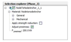
Figure 2-5: Node-to-node anchor in the Selection explorer
