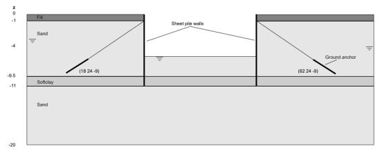
Figure 2-2: Cross section of the excavation pit with the soil layers
