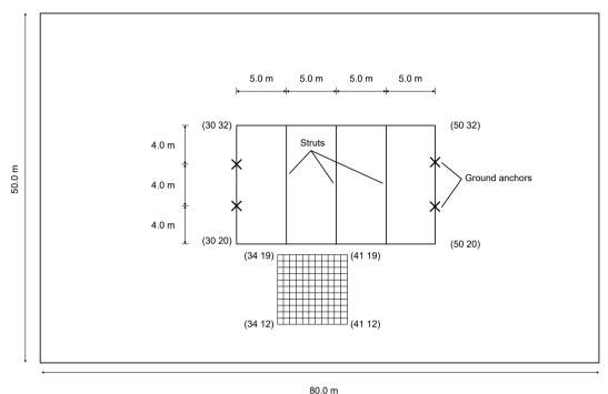
Figure 2-1: Top view of the excavation pit
