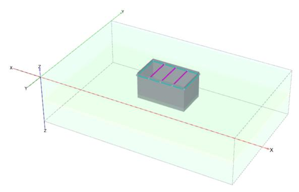
Figure 2-3: Visualization of struts and walings - Structures mode
